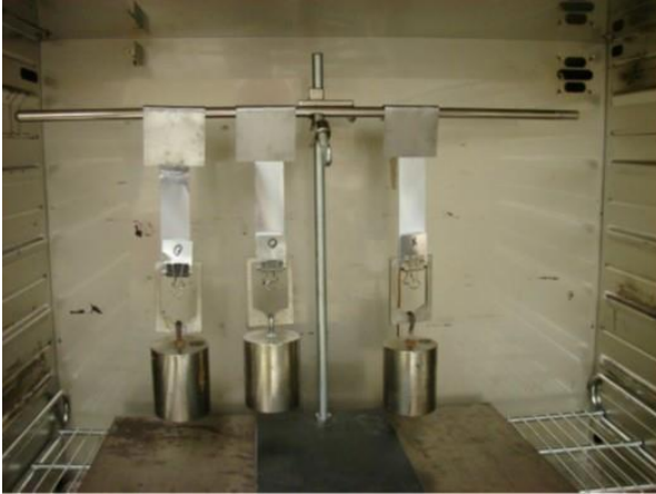
Fig.10. Oven testing of adhesive before lamination for minimum drift.
